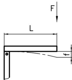
$$f [\text{mm}] = \frac{0.476 \times F [\text{N}] \times L^3 [\text{m}]}{I [\text{cm}^4]}$$
