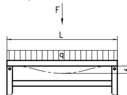
$$f [\text{mm}] = \frac{0.0037 \times F [\text{N}] \times L^3 [\text{m}]}{I [\text{cm}^4]}$$
