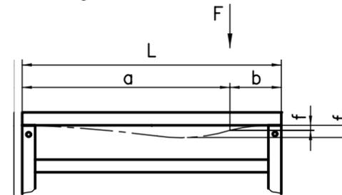
$$f [\text{mm}] = \frac{0.476 \times F [\text{N}] \times a^2 [\text{m}] \times b^3 [\text{m}]}{I [\text{cm}^4] \times L^3 [\text{m}]}$$
